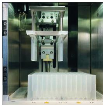
Deep-well plate for processing up to 16 samples
